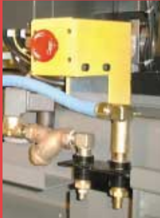
Closed-loop feed throat temperature control Standard on all units
